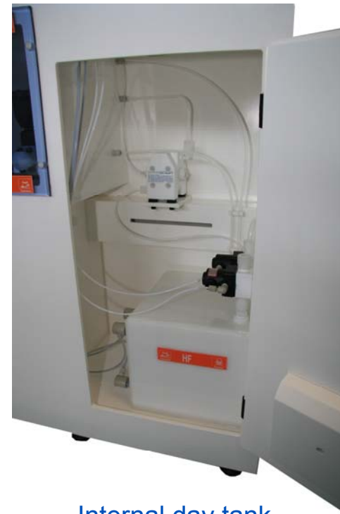
Internal day tank (model with chemical filling from CDS)
